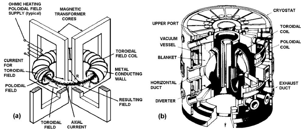
FIG. 17.12. (a) The torus magnetic confinement principle. (b) Schematics of the JET (or ITER) tokamak experimental reactor.
