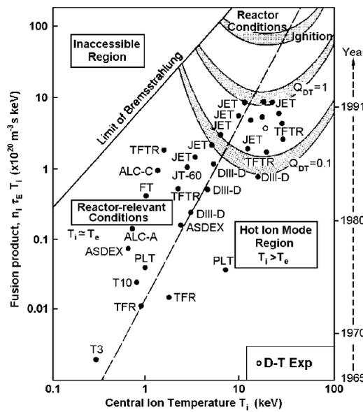
FIG. 17.13. Results obtained by different fusion reactor designs.
