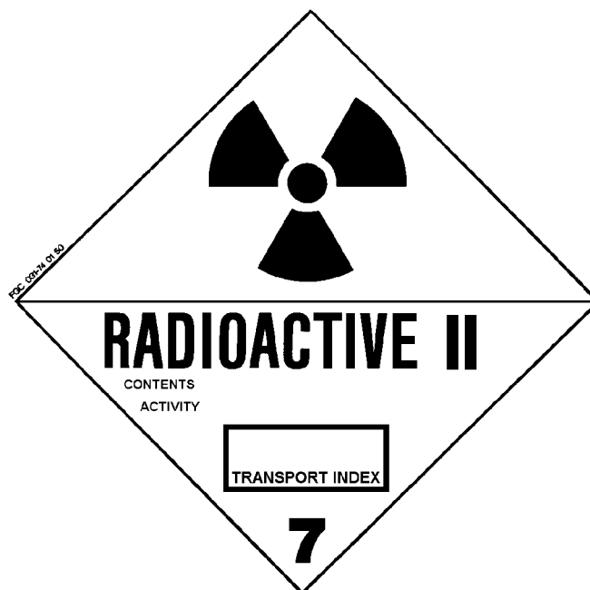
FIG. 18.13. Label for shipment of radioactive material of class II. "II" in red with a yellow background.
