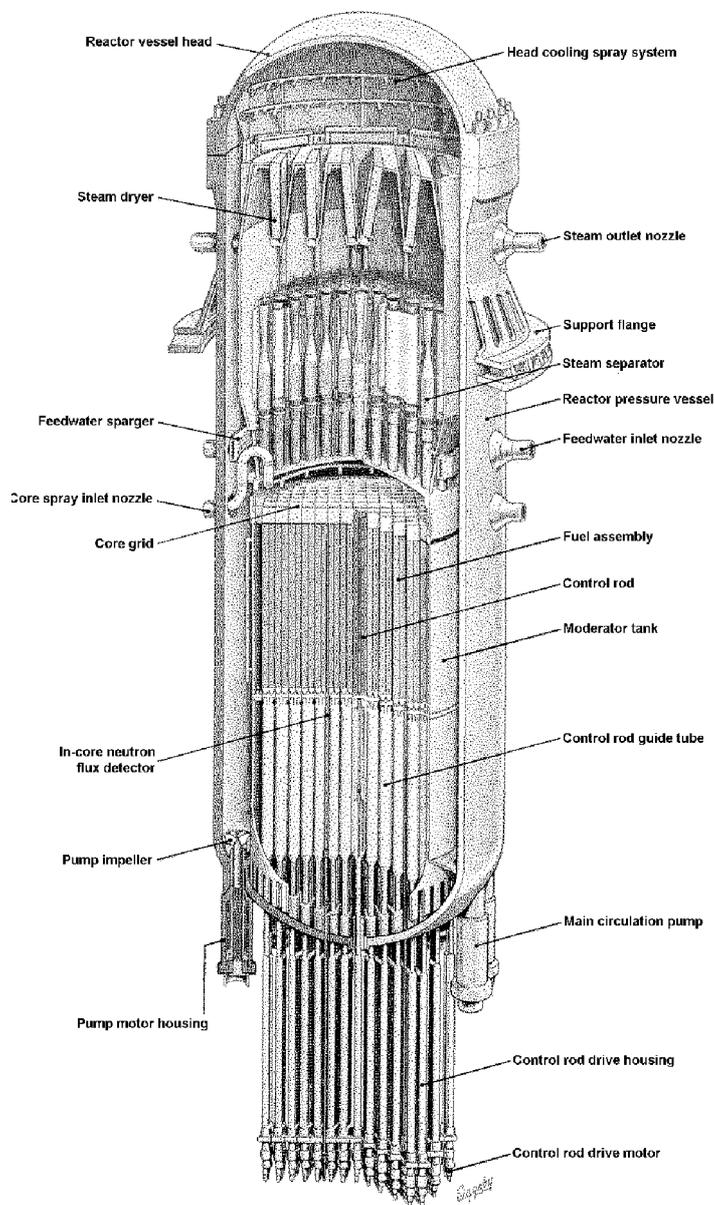
FIG. 19.13. Design of a boiling water reactor core system, ABB-Atom, Sweden.
