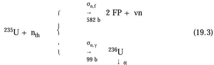
$^{236}\text{U}$  decays through  $\alpha$ -emission. Due to its long half-life ( $2.3 \times 10^7$  y) it accumulates in the reactor.  $^{236}\text{U}$  may capture a neutron, forming  $^{237}\text{U}$ , which over a few days time decays to  $^{237}\text{Np}$ . The *neutron yield per fission*,  $\nu$ , is an average value which depends on the neutron
