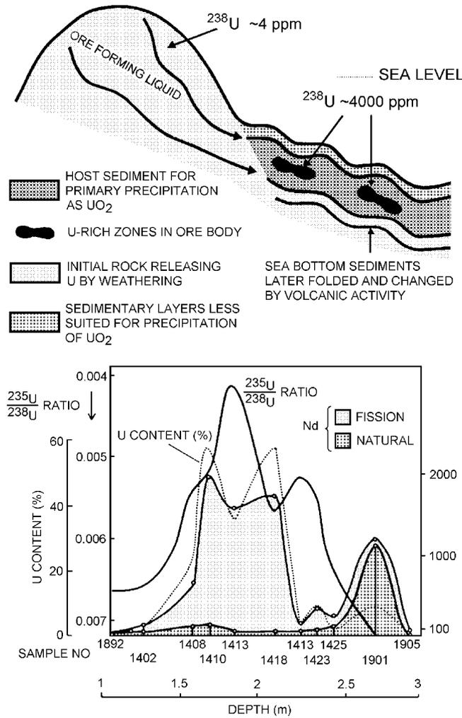
FIG. 19.10. Schematic view indicating the formation of the Oklo ore deposit and some data on its current local composition.
