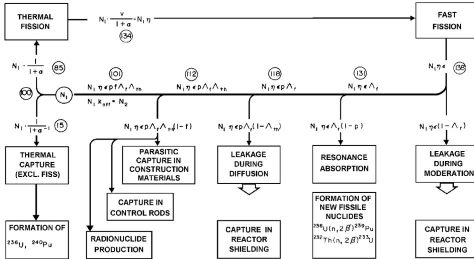
FIG. 19.6. The neutron cycle in a thermal reactor. The number of neutrons for 100 in first generation are given in circles (data from an old Belgian research reactor, BR1).
