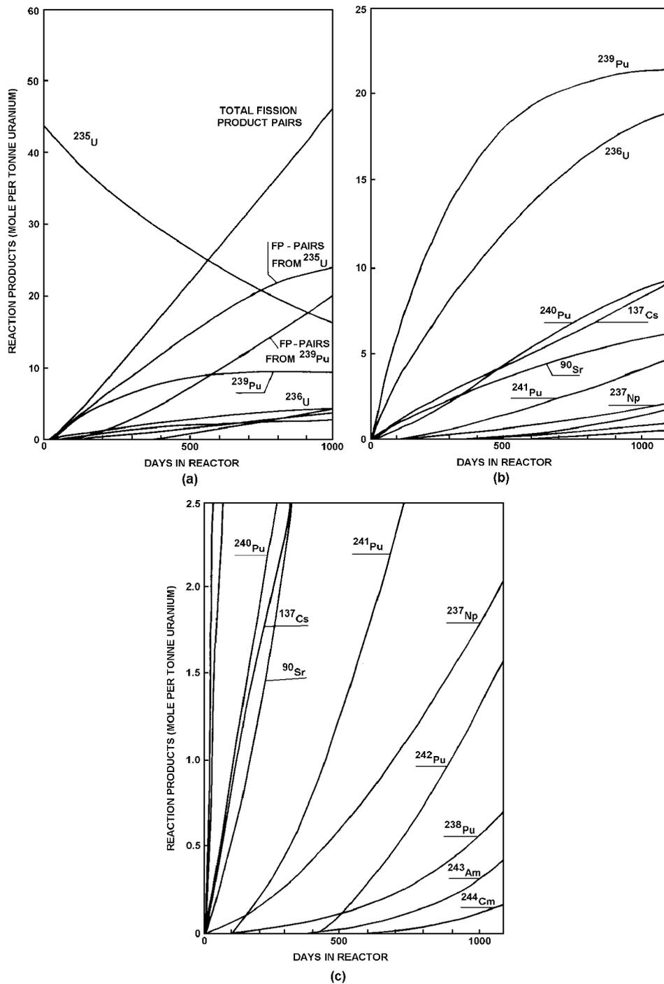
FIG. 19.7. Build-up of reaction products in fuel originally enriched in  $^{235}\text{U}$  to (a) 1% used in a graphite reactor ( $\sim 230 \text{ MW}_{\text{th}}$ ), (b) and (c) 3.3% used in a LWR ( $\sim 1000 \text{ MW}_e$ ).
