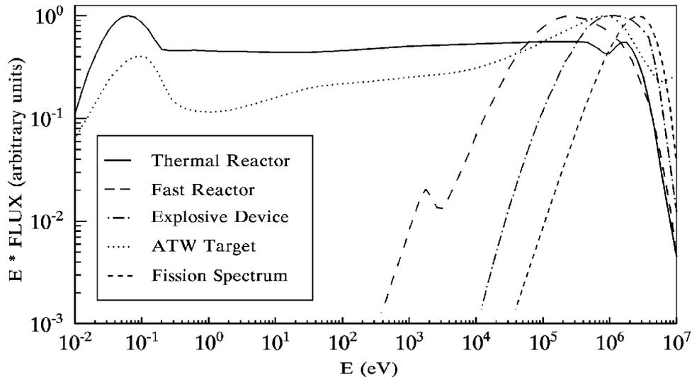
FIG. 19.4. Neutron spectra of some chain reacting systems and a proposed accelerator driven system. The abscissa shows neutron flux times energy on an arbitrary scale.
