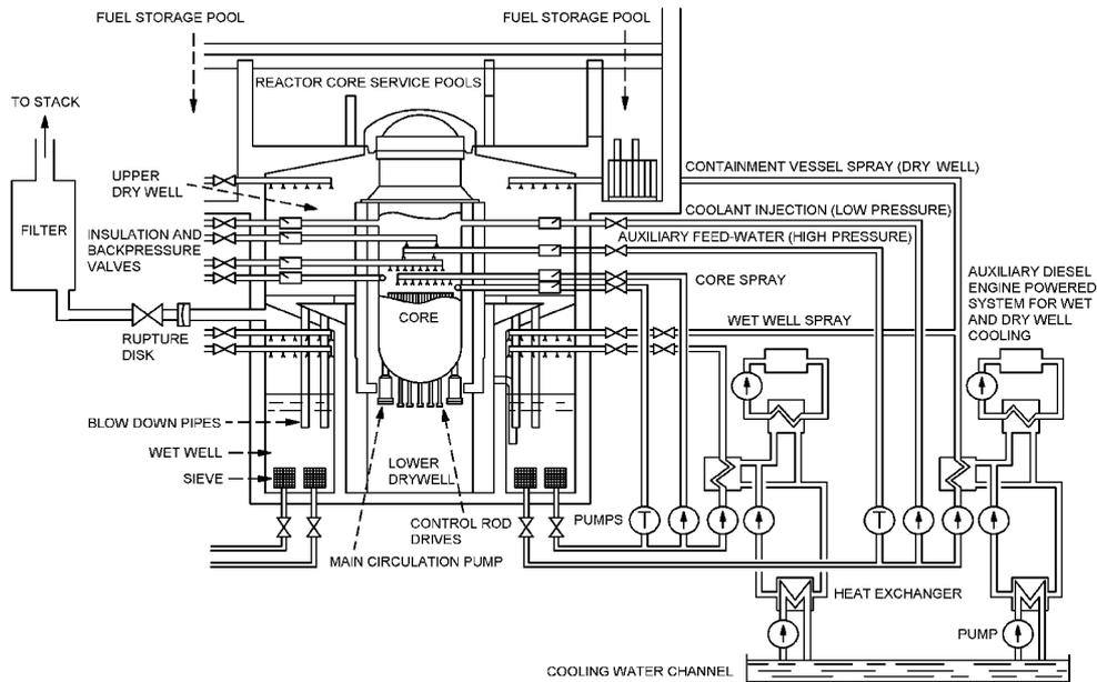
FIG. 19.16. Emergency cooling and pressure relief system of ABB-Atom boiling water reactor (only one half of the cooling system is shown).
