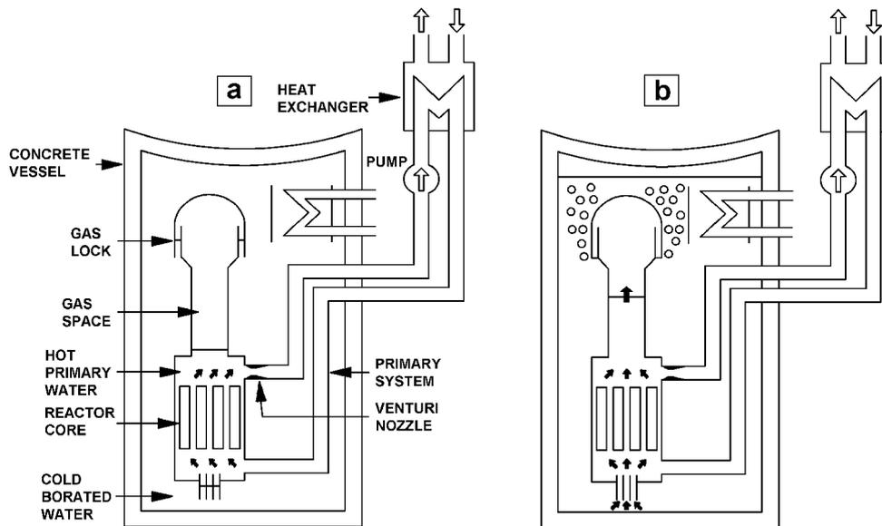
FIG. 19.14. Working principle of ABB-Atom SECURE inherently safe district heating reactor.
