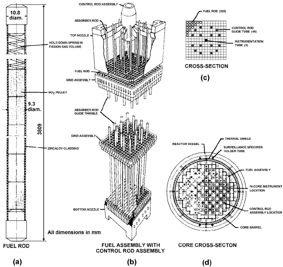
FIG. 19.12. Typical PWR fuel pin (a), assembly (b, c), core (d), and vessel (e) designs.
