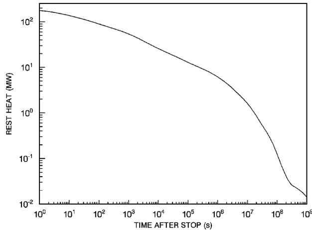
FIG. 19.15. Decay heat from a 3000 MW<sub>th</sub> LWR core, which has been operated continually for 300 days, as function of time after shutdown.
