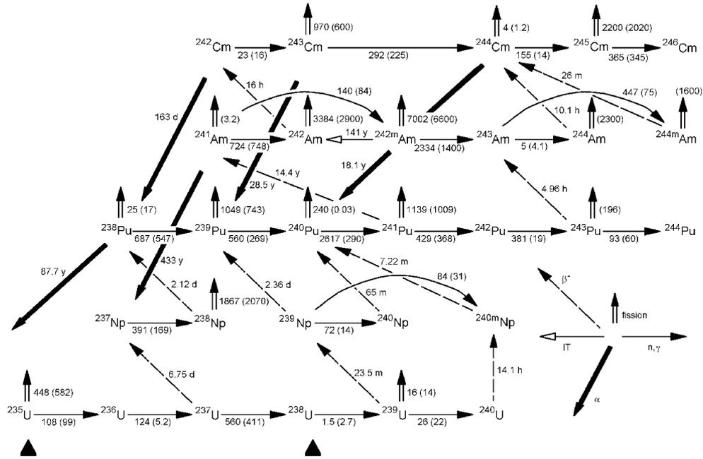
FIG. 19.5. Nuclear reactions in irradiation of uranium. Figures along the arrows are half lives or effective cross-sections (b) for a typical power LWR, with thermal (0.025 eV) data within parentheses.
