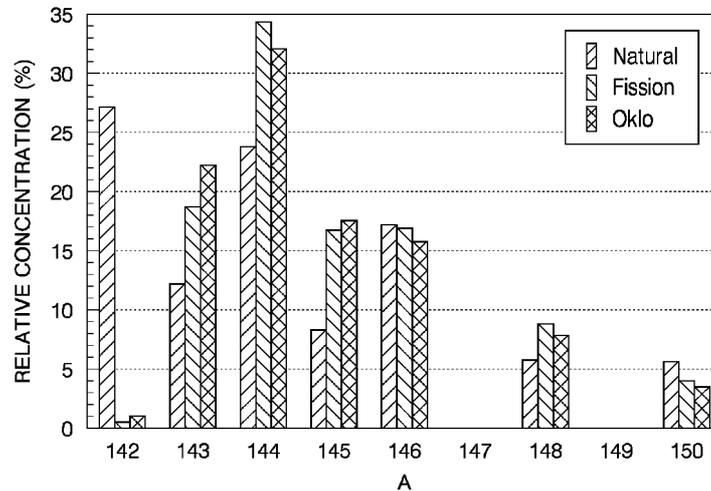
FIG. 19.11. Comparison of the isotopic composition of neodymium from normal Nd ore, from  $^{235}\text{U}$  fission in a BWR and from Oklo.
