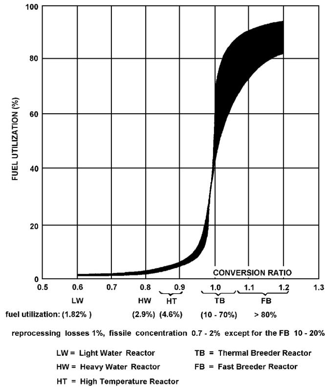
FIG. 19.9. Conversion ratios and fuel utilization efficiencies. (From Thermal Breeder Consultants Group, Salzburg, 1977.)
