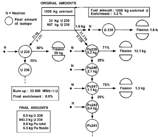
FIG. 19.8. Fission product balance in a light water power reactor. (From F. Hoop.)
